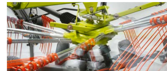
Cardanic rotor suspension ensures that the rotors follow the ground contours independently of the tractor.
