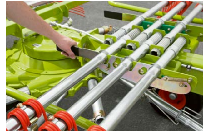
With some models, the tine arms have to be removed for road transport – but they can be stowed away in no time at all.
