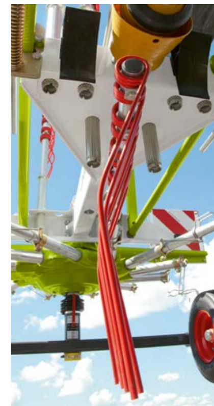
The 9 mm thick standard tines on the 450, 420, 370 and 320 models are extremely robust, making them ideal for both hay and silage.
