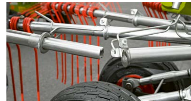
Lemon profile attachment and PROFIX tine arm bracket in the LINER 700.
