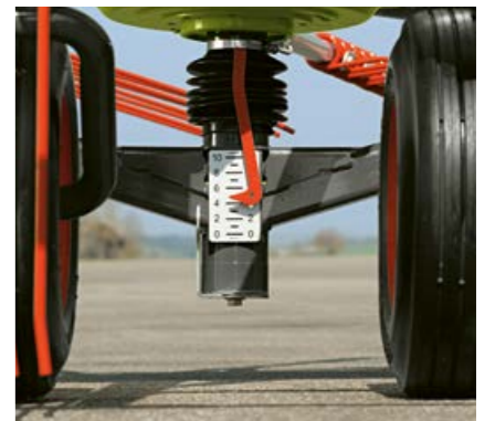
Keeping it flexible, with the rake height adjustment scale.
