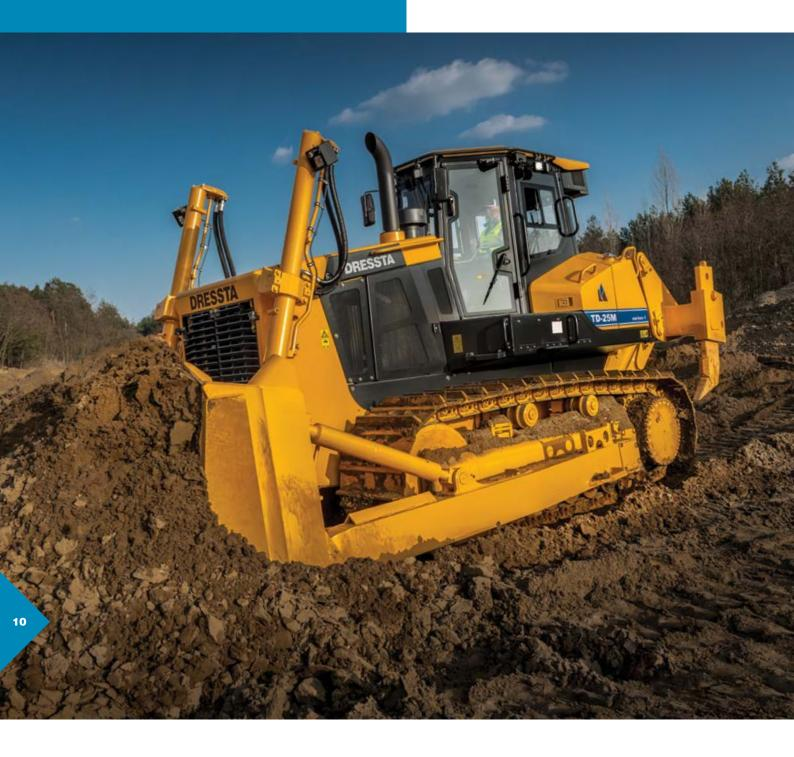
A massive one-piece frame, high strength pivot shaft and exclusive undercarriage design provide maximum durability and suspension while giving the operator a smooth, stable ride.
