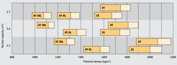
HT = Standard height arm HT HL = High lift arm HT SHL = Super high lift arm ZX = Z-bar
