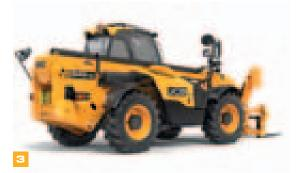
Most Tier 4 Final / Stage IIIb engines use a Diesel Particulate Filter (DPF). EcoMAX doesn't, so there's no loss of productivity during the regeneration process, nor the extra expense of replacing a DPF.
