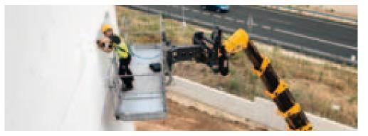
Further widening the versatility of the JCB Loadall, the aerial work platform is more mobile and cost effective than a boom or scissor lift.
