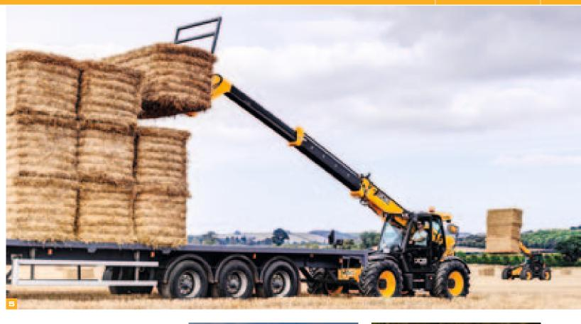
Innovative all-new smart regenerative hydraulics helps to make the most of every drop of precious fuel. Gravitational forces are harnessed to make boom lowering and retraction more energy efficient than ever.
